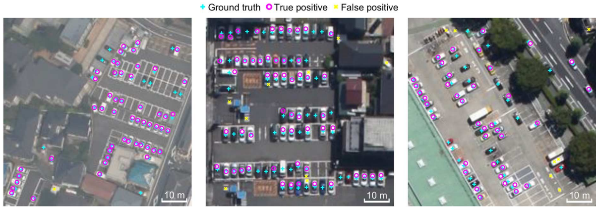
Fig. 5. Car detection results for three test images obtained by SR-Hough at precision = 0.896 and recall = 0.754.
